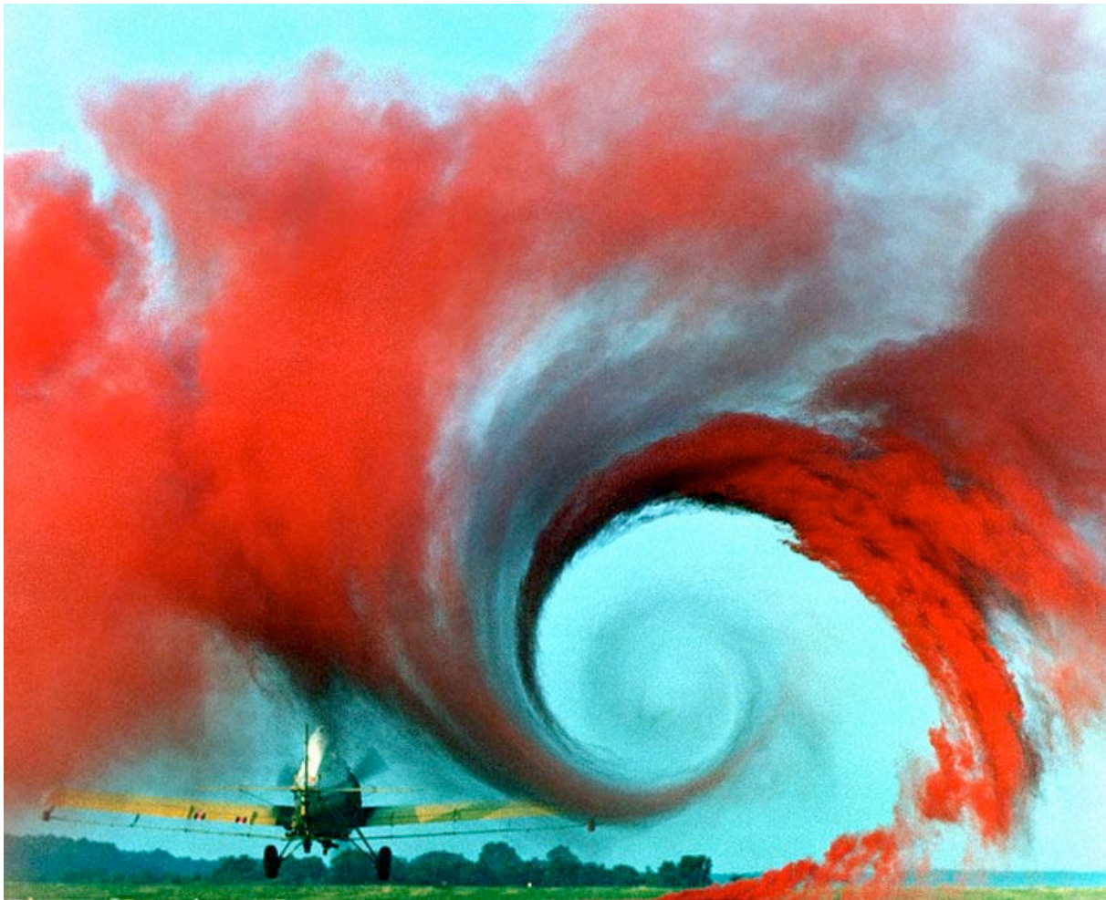
Vortex created by the passage of an aircraft wing, revealed by colored smoke.
